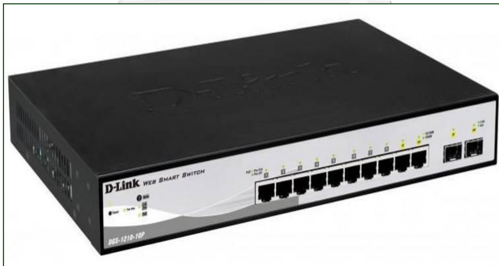
Figura 34: Switch DGS-1210-10P-Dlink (8-ports Gigabit - 2-ports Combo UTP/SFP; PoE Smart Switch) (Fuente: www.dlinkla.com )
